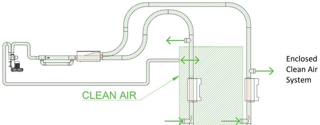
Alternatively, we can design a fully enclosed clean air system with through type stations only and tubed in clean air. Other variations are available including fine filtering air.
