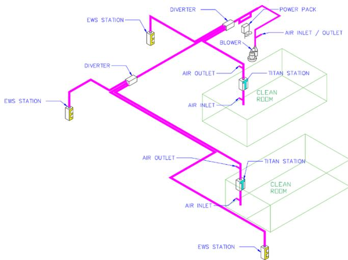
Delivering samples or other small items by foot to a clean room in a processing plant poses several problems with infection control protocols and can also be a time consuming, repetitive walk to and from the sampling area to the sterile area crossing infection control borders.
