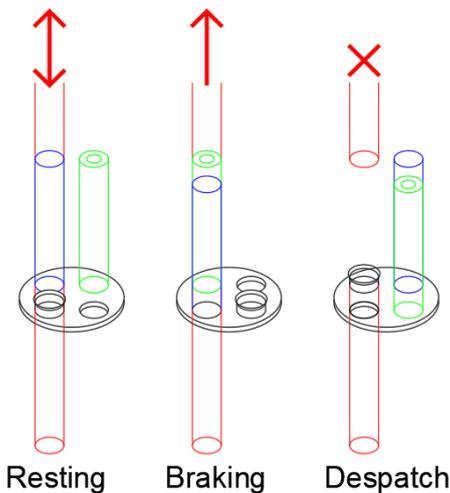
The unique rotating design of the Titan Station is ideal for clean room application as the tube is continued through the mechanism therefore air is contained.
